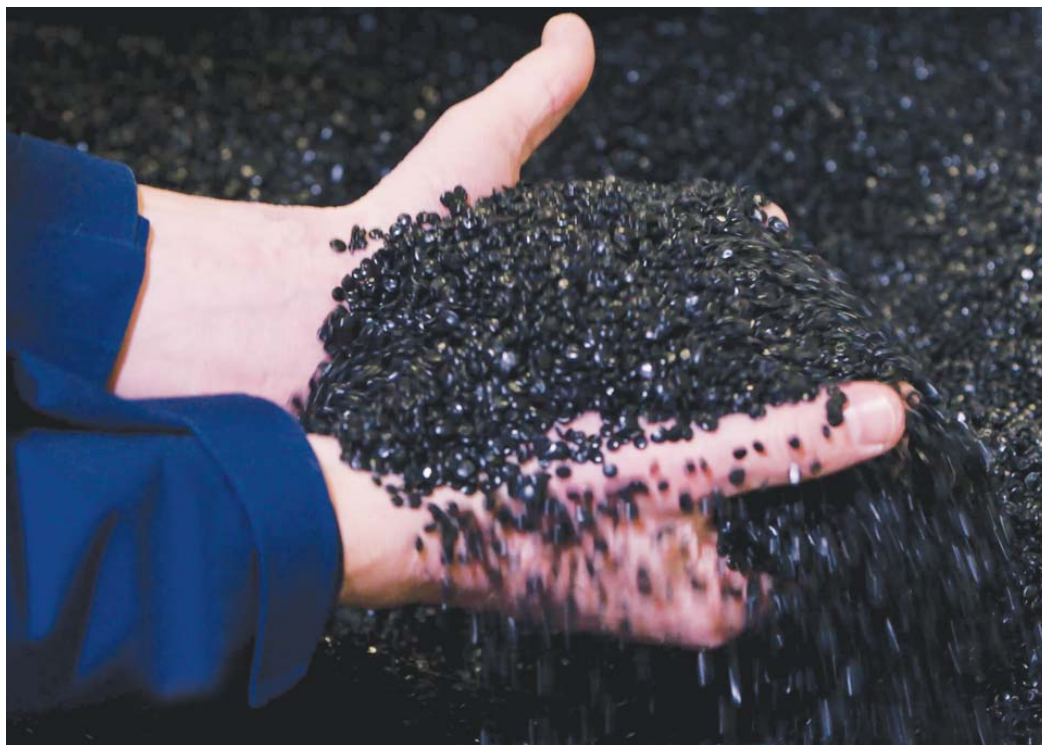
Figure 7 – Regranulated material ready for reintegration into new product manufacturing.
