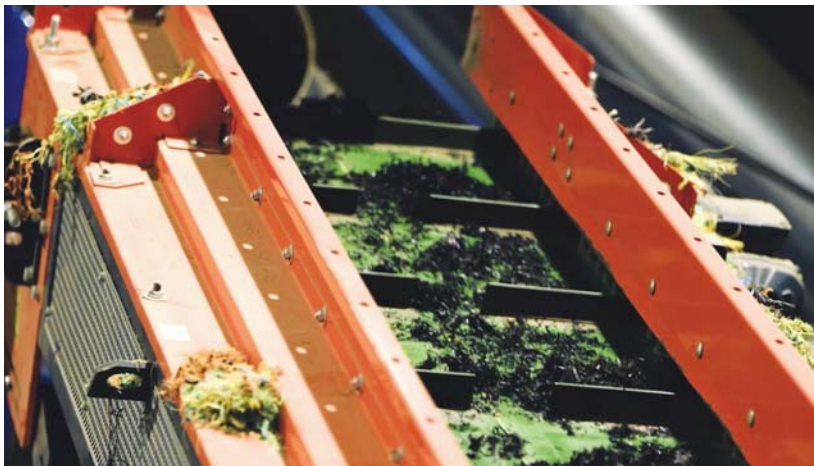
Figure 5 – Shredded geotextile material prepared for the washing and recycling process.
