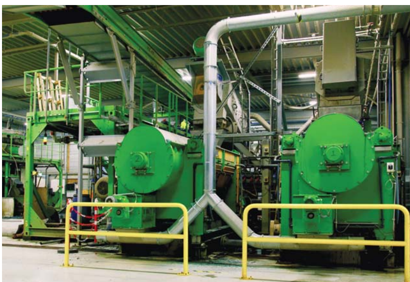
Figure 6 – Washing stage of shredded geotextile material to remove embedded soil.
