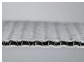
Drain made of recycled polymer
