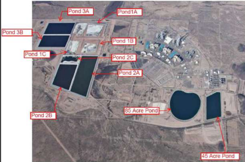
Figure 2 from Eichelberger – Palo Verde Electrical Generating Station near Phoenix AZ. (For scale the three blue rectangular buildings are nuclear reactors.) All ponds pictured were lined with white materials totaling appx. 310 acres/1.25 square km.
