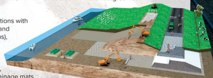
Schematic overview of the use of geosynthetics in flood defences with geosynthetic clay liners, soil reinforcement, nonwoven geotextiles for filtration/separation and erosion protection on embankments.
