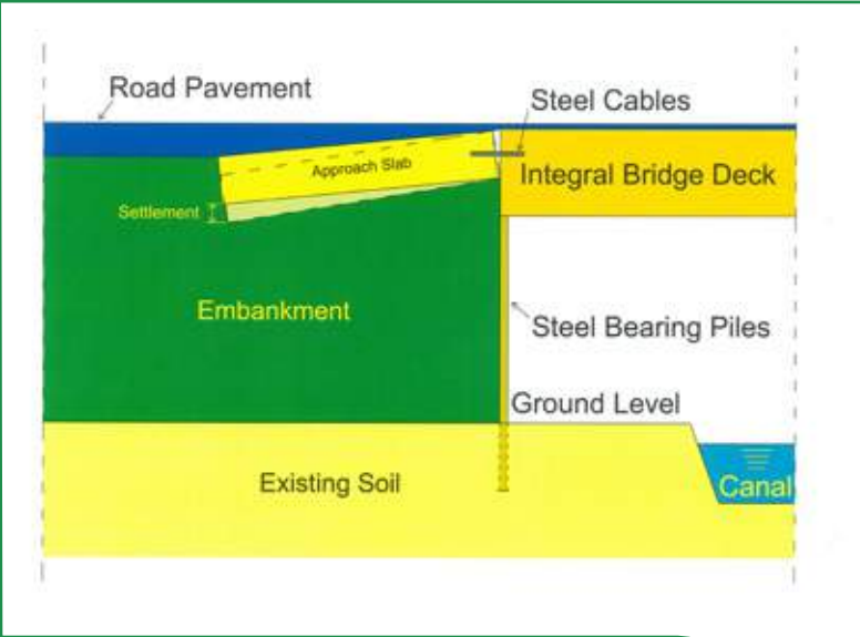
Figure 2 - Explanation of the function of an approach slab
