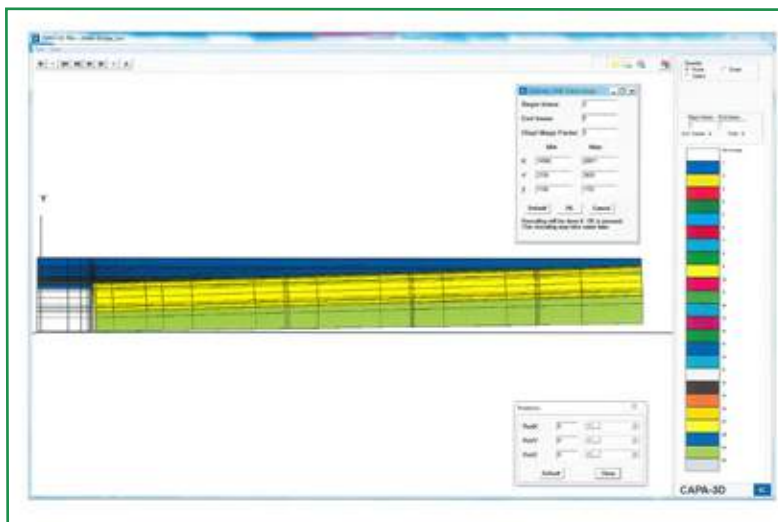
Figure 4 - Detail mesh, focussed on the important locations
