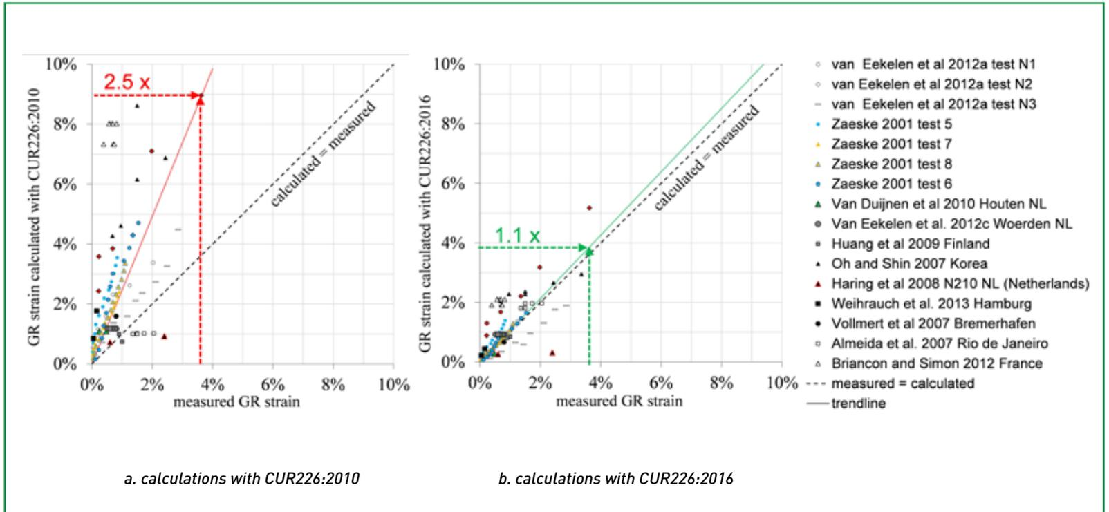
**Figure 3** - Comparison calculations and measurements in seven field projects and four series of experiments. Van Eekelen et al., 2015 gives the sources of the references given in this picture, which are not given in the references of this paper due to space limitations. Calculations without safety factors.
