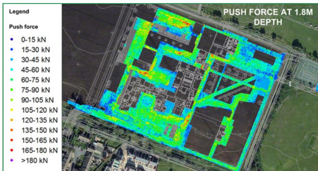
**Figure 2 -** Map showing the push force at a specific depth in a highly optimized and complex installation grid, only possible to execute with GPS based logging and positioning.
