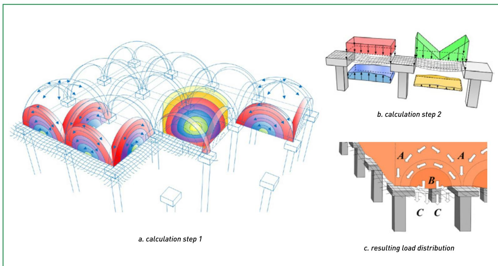
**Figure 2** - The new Concentric Arches model (Van Eekelen, 2015 and Van Eekelen et al., 2012b, 2013, 2015) consists of two steps: (a) step 1 calculates the load distribution in A and B+C and (b) step 2 calculates the GR strain that occurs in the GR strip between adjacent pile caps (c) resulting load distribution (A, B, C).
