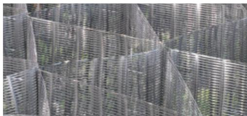
Figure 1 - 3D Geocell structure
