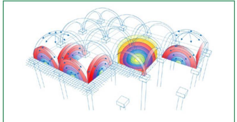
**Figure 2** - Concentric arches in a piled embankment.
