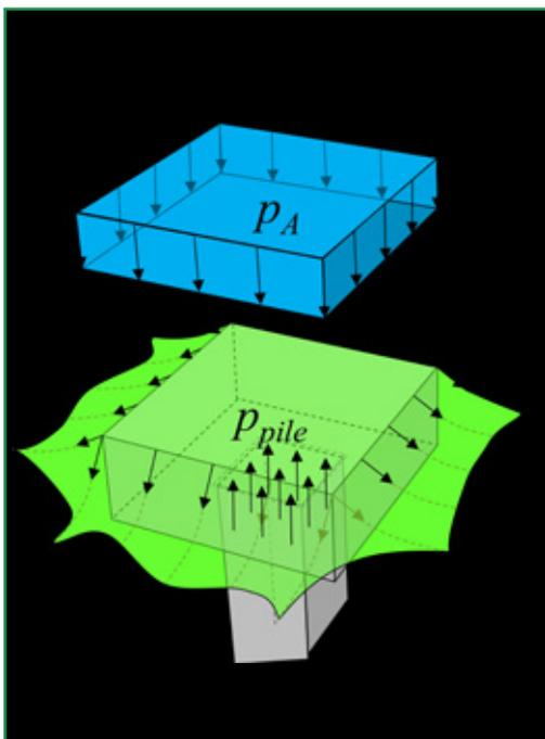
**Figure 5** - Loads on a pile cap: arching  $p_A$  (kPa), the tensile force  $T$  (kN/m) and the axial pile force  $p_{pile}$ , uniformly distributed (kPa).
