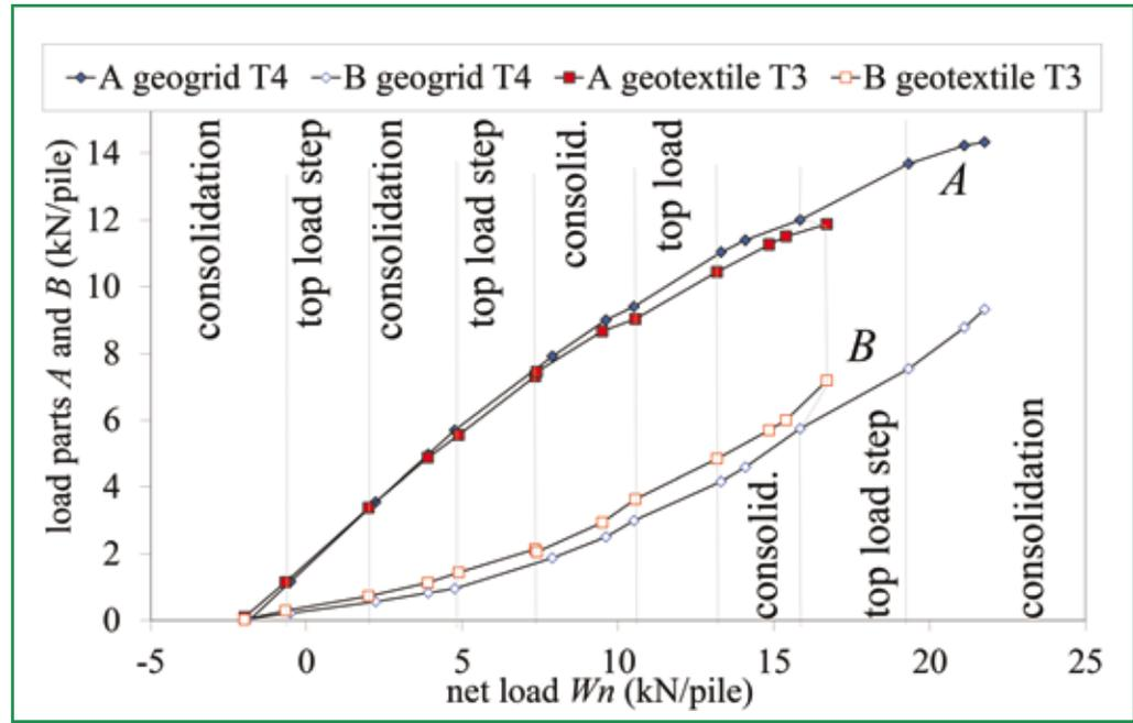
Figure 1 - load transmitted to the piles (part A) and to the geosynthetics (Part B).
