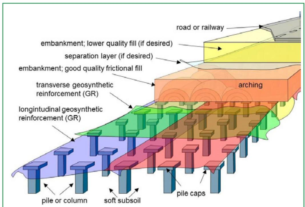
Figure 1 - A basal reinforced piled embankment.
