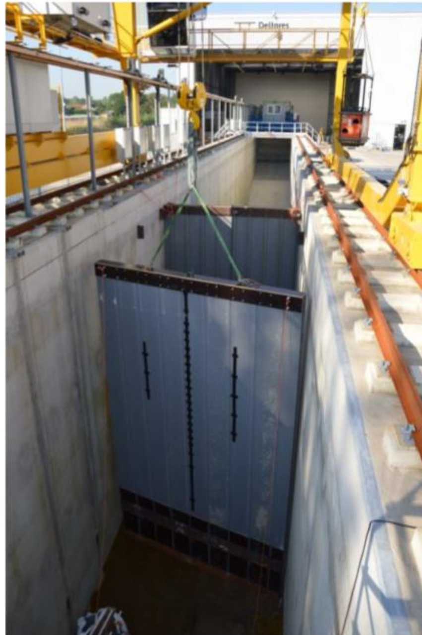
Figure C.12 Installation of the front wall in the flume
