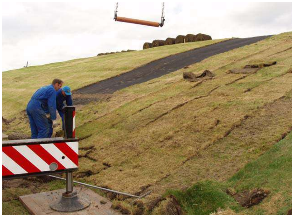
Figure 3-9: Replacement at the primary test section (without manual repositioning and removal of overlaps)
