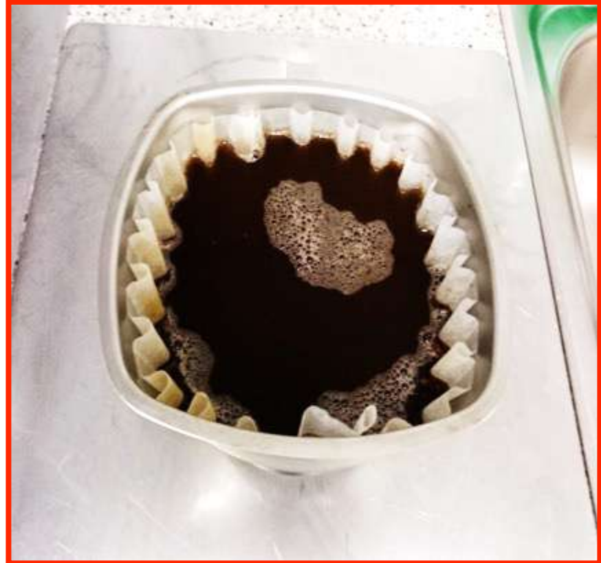
Hydraulically unstable filter (clogged/blinded)
