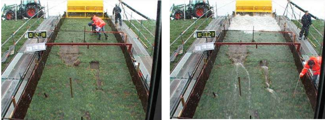
Figure 9-8: Start of the gully formation downstream of the damaged areas
