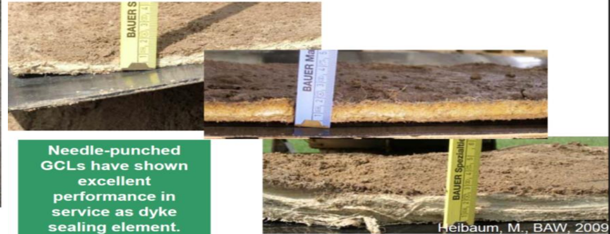
GCL excavations 2008 - 4, 6 and 12 years in service
